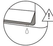
Caution: Do not keep the louver at too vertical an angle for long periods of time. This can cause water condensation to drip on your furnishings.
